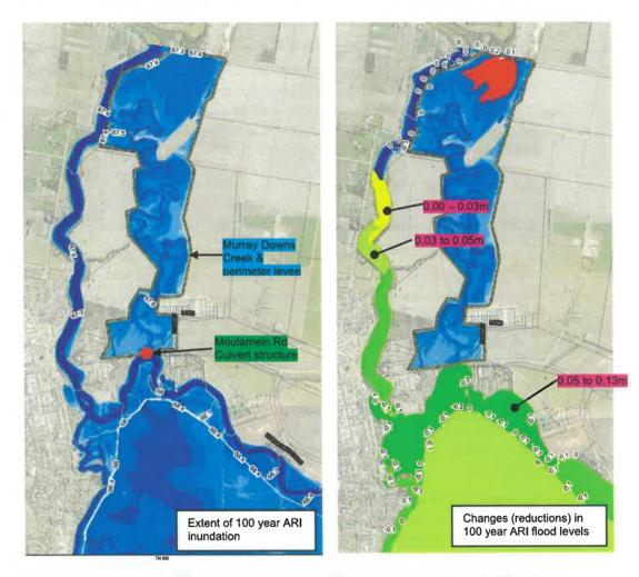
Figure 11 Hydraulic ModellingResults - Murray Downs Creek Floodway
